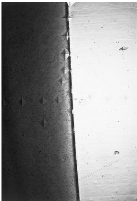
Figure 3 Micrograph showing indentation on the surfaces of the injection molded plate near the weld line area (see Fig. 1).
